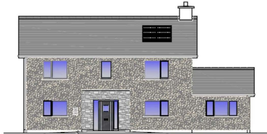
FRONT ELEVATION HOUSE TYPE 6 SCALE 1:30
