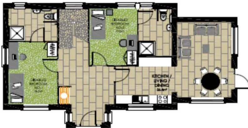
GROUND FLOOR PLAN HOUSE TYPE 6 SCALE 1:30 GROUND FLOOR PLAN AREA = 143.7sq.m
